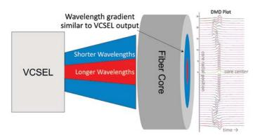
FIGURE 2 – Side view of VCSEL spatial-wavelength characteristic and wavelength gradient in fiber core when well aligned
