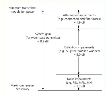
FIGURE 1 – Typical power budget for 25G and 100G Ethernet over MMF
