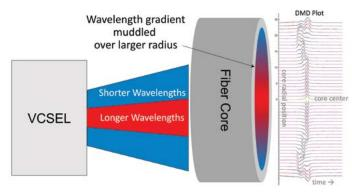
FIGURE 3 – Side view of VCSEL spacial-wavelength characteristic and wavelength gradient in fiber core when not well aligned
