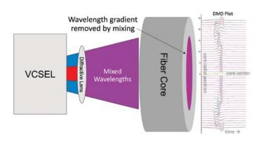
FIGURE 4 – Diffractive optic mixes wavelengths removing gradient in fiber
