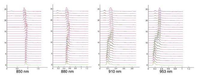
FIGURE 6 – DMD plots of OM5 fiber for wavelengths spanning both BiDi and SWDM4 applications.
