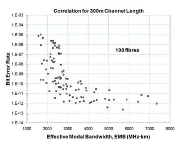
Figure 2. Bit error rate at -11.0dBm receive power for 100 fibers verses fiber effective modal bandwidth. The data shows poor correlation.
